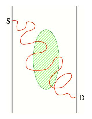
**Problem:** Reconstruct the optical absorption from boundary measurements.
